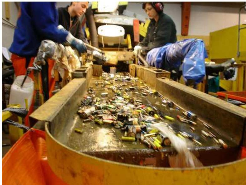
**FIGURE 1: MANUAL BATTERY SORTING**
