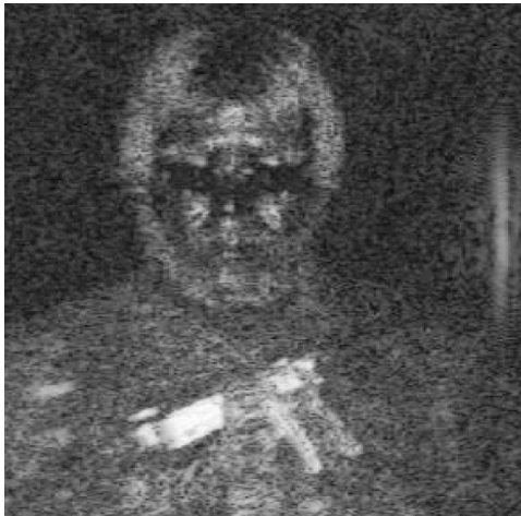
Figure 2: Active image showing reflected power from a person with a handgun hidden under a shirt, taken at 640 GHz[2].
