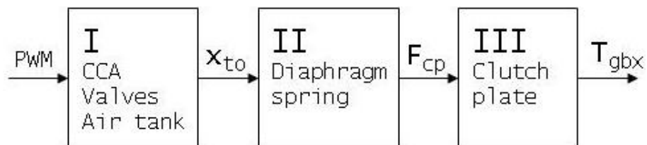
Figure 3.1: How the clutch system is divided and structured into three parts.
