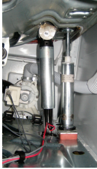
Figure 11: The semi-active damper mounting seen from the back of the machine
