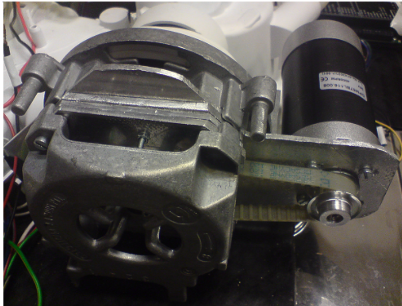
Figure 19: The gearbox, connects the pump-shaft inside the old motor-housing to the left with the new DC motor to the right with a reduction of 28:19
