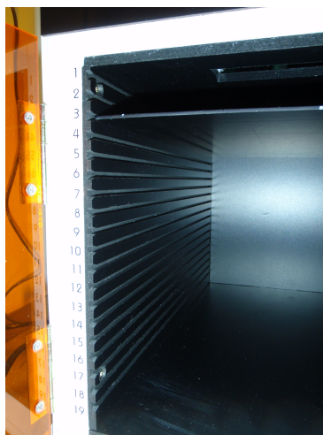
Figure 4.3 - Inside the UV light exposure device there are a scale of steps, with different highs from the UV source, where the discs can be placed.
