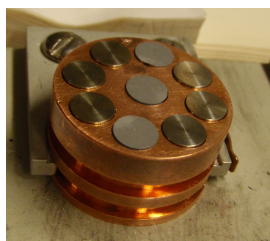
Figure 5.4 - A specific rack for the XPS study where the discs are placed on. The diameter of one disc is 6 mm and of the rack around 30 mm.
