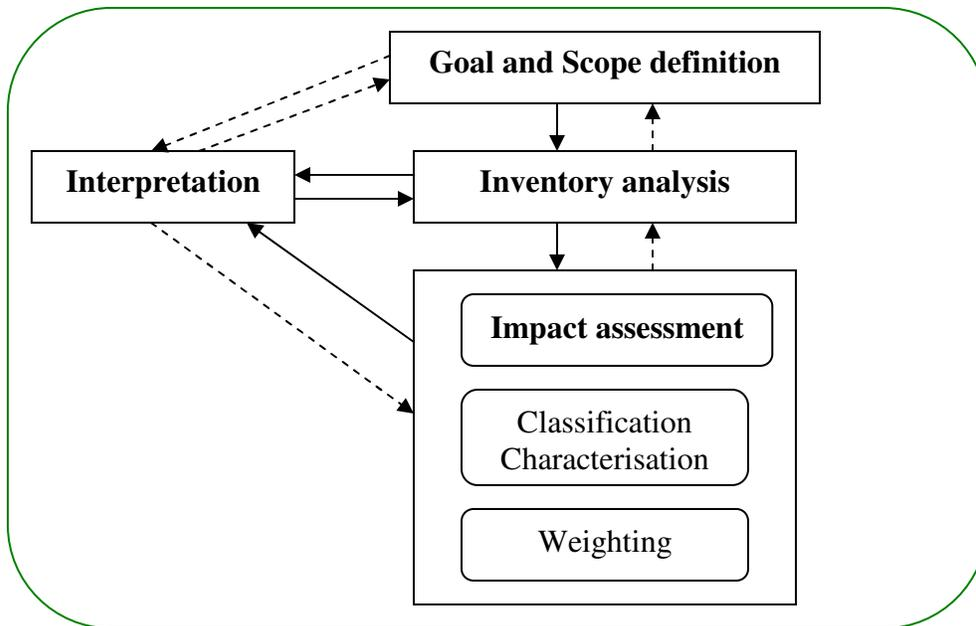
**Figure 1.2 The LCA procedure (from Baumann and Tillman)**
