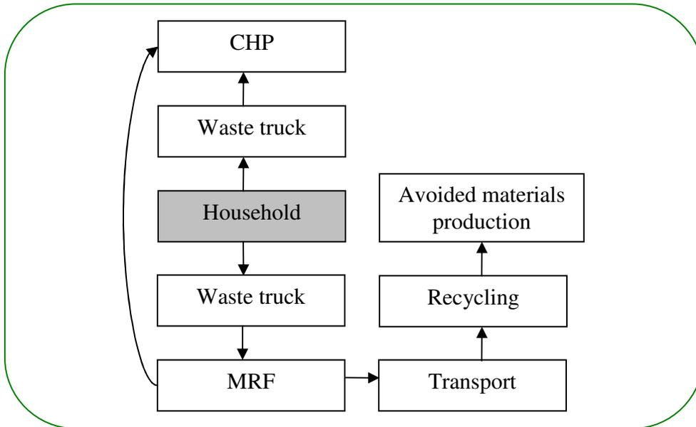
**Figure 3.2 Simplified flowchart of the Co-mingled collection system.**
