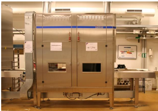
Figure 3.1. The IR oven at SIK. The section to the right has short IR waves and the section to the left has medium IR waves.
