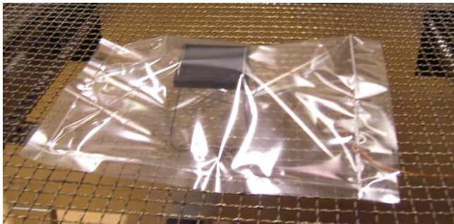
Figure 3.8. The black body inside a plastic pouch. The pouch is sealed with an impulse sealer and one small hole was made in the plastic pouch to let the water steam out because steam needs a larger volume than air.
