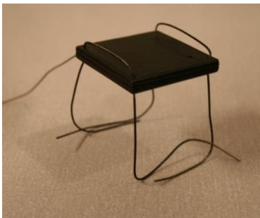
Figure 3.3. The black body setup with legs rises the black body around 5 cm from the grid. The black body is connected to the memory logger with a thermocouple.
