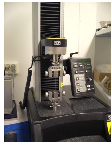
Figure 3.4. Tensile tests were performed on an Instron Universal Testing 5542 in a climate room holding 23 °C and RH 50%.
