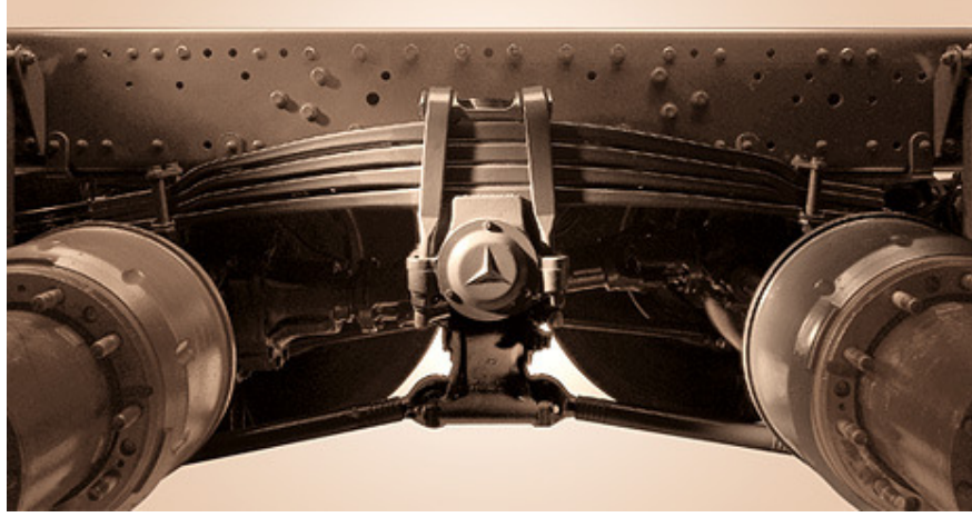
Figure 9 A tandem axle construction by Mercedes (Adopted from Ref. [21]). The axle group is able to pivot with the help of rotating joint where the brand badge is located.
