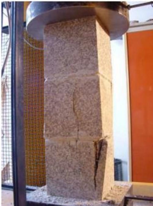
Figure 6.2 Test of compressive strength for granite prisms joined with soil mortar. Vasconcelos G. et al. (2009)
