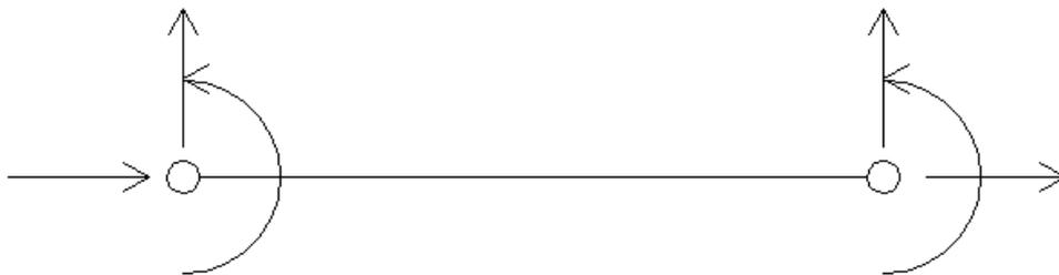
Figure 4.5 Beam element with six degrees of freedom.
