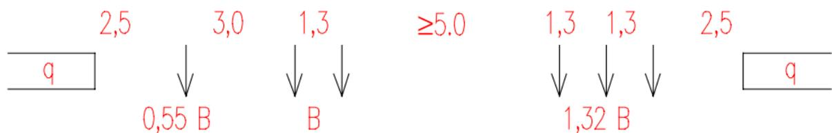
Figure 7.2 Design code vehicle h). Vägverket (1998)
