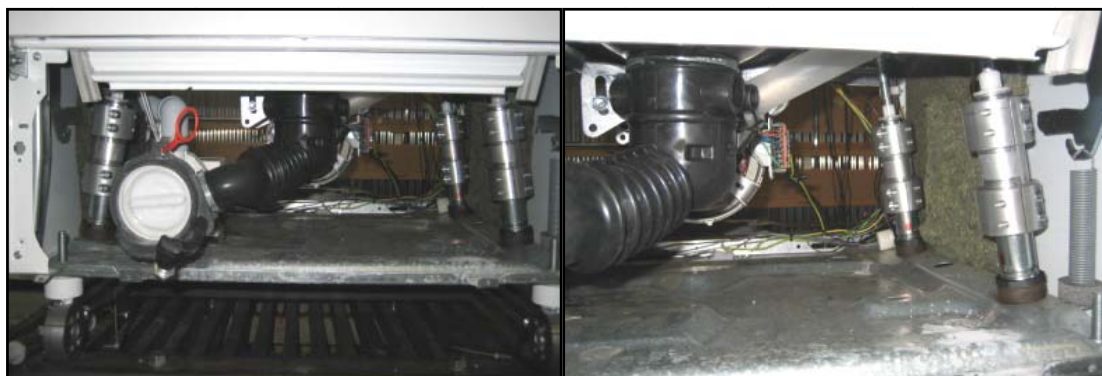
Figure 5.3.2 Prototypes mounted in the washing machine test rig
