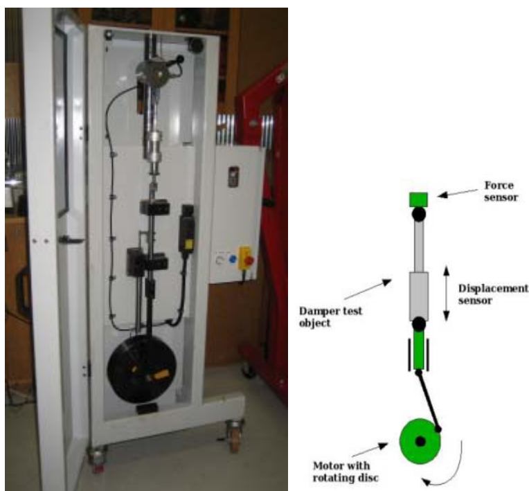
Figure 5.1 Damper test rig and sketch. Extract from [29]
