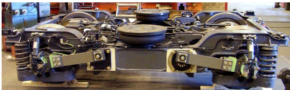
Figure 5.1: Reference photo of the bogie used in high speed trains.
