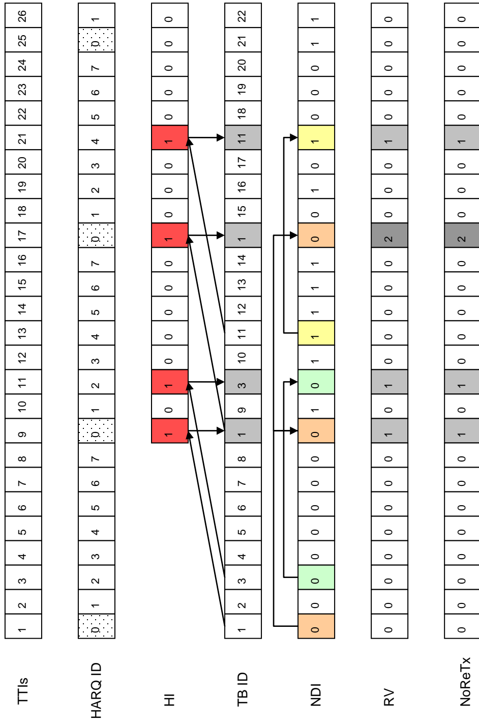
Figure 3.31 The HARQ processes of the simulator (QPSK).
