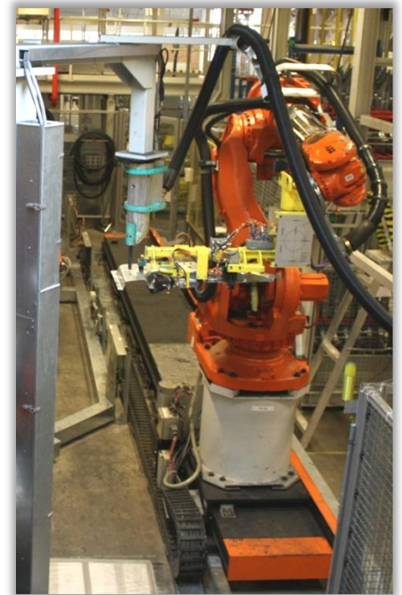
Figure 3 – ABB Robot applying glue on a metal part in station 15-38-110
