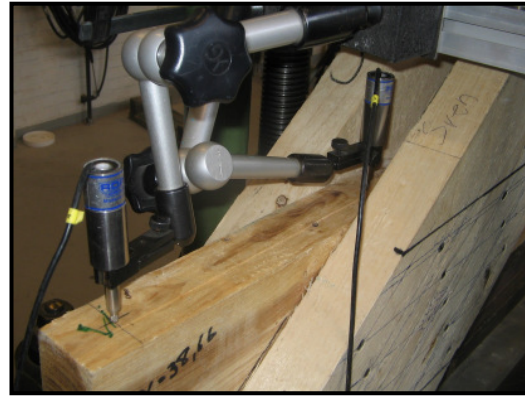
b) Setup of LVDT above rotational centre and the end of the truss
