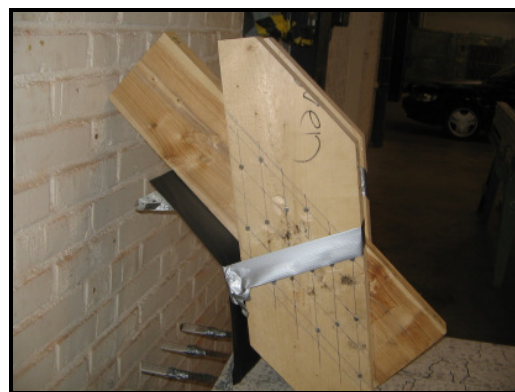
b) Fastening of image plate (bowed)
