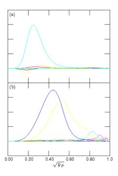
Figure 5: Radial structure of the modes found numerically with MISHKA-1. Upper figure: Core-localized cascading mode with  $q_0 = 0.95$ . Lower figure: Tornado-like TAE with  $q_0 = 0.91$ . Both modes have toroidal mode number n = 6.
