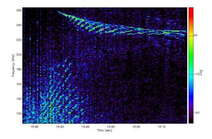
Figure 2: Magnetic spectrum prior to a monster sawtooth crash, as measured by O-mode interferometry. Both sweeping up modes and tornadoes are clearly visible.
