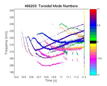
Figure 1: Magnetic spectrum obtained by Mirnov coils outside the plasma, showing tornadoes and their mode numbers just before the monster sawtooth crash at t = 11.3 s.
