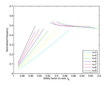
Figure 4: Frequency evolution of the modes found numerically with MISHKA-1, as a downward sweep from  $q_0 = 1$  is performed.
