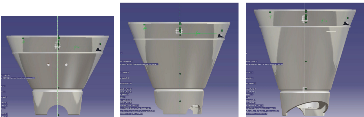
Figure 6.38 The Cone front ring on different lamp housings
