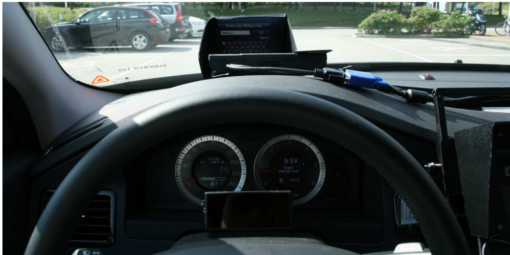
Figure 12 Head up display substitute for Remote View experiment (also rectangular enclosure of the eye tracker can be seen in front of instrument cluster).
