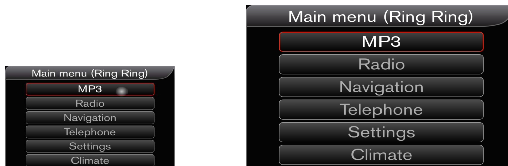
Figure 8 Example of the static RV (RVs) view on the HUD and on the TS.
