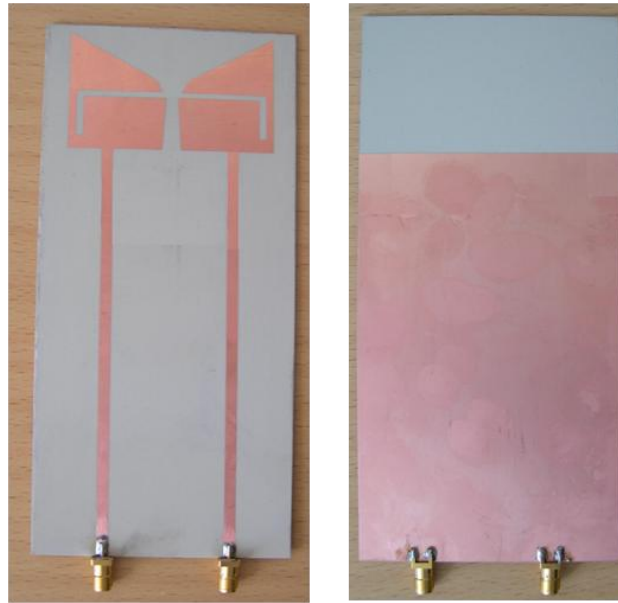
Figure 3.8 Prototype of the designed MIMO/diversity antenna: (left) top view, (right) back view.
