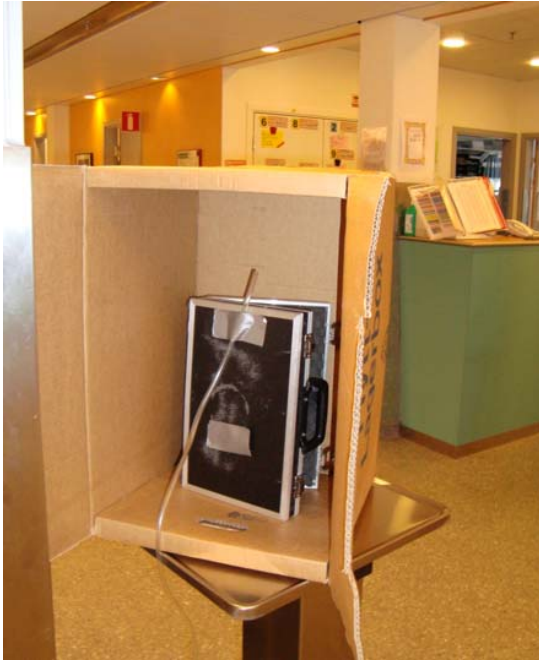
Figure 5.7 End of second tube placed in a box in the corridor to avoid vortices created by movements that would affect the outcome.
