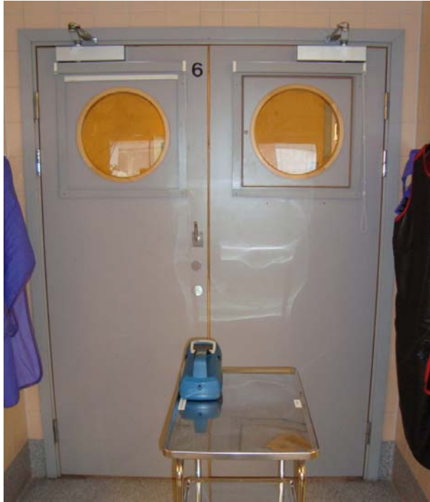
Figure 5.9 P-TRAK placed on a table in the operating room to measure the increase of particles due to door openings. The device was located at varied distances from the door.
