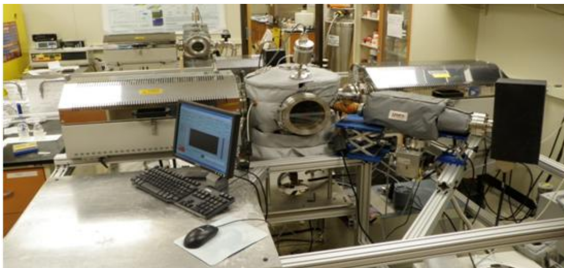
Figure 10. The two-source CVD system used for gradient manufacturing
