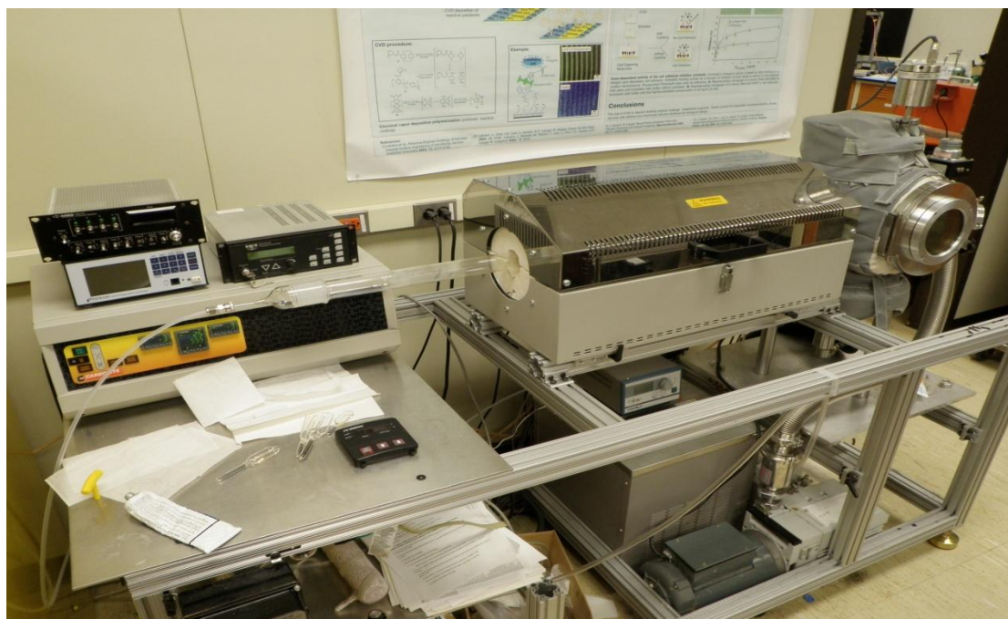
Figure 9. The one-source CVD used during the project
