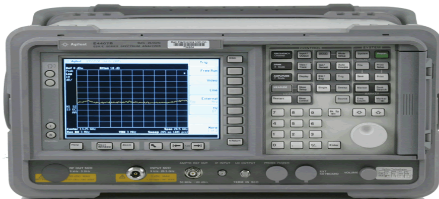
Figure 2.3: Agilent E4407B Spectrum Analyzer [6].
