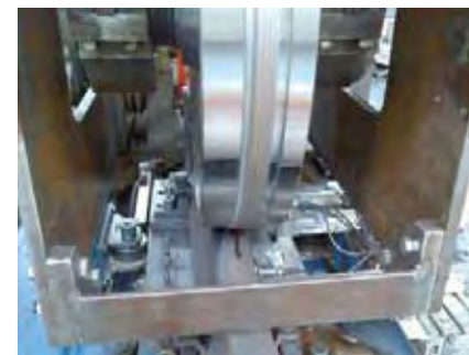
Figure 6.1.4-1: Test rig for frog materials at DB in Kirchmöser (left) and test specimen (right)
