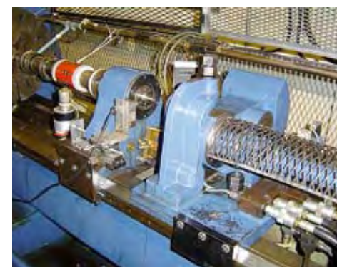
Figure 5.4.1-1: Left: twin disk test rig (SUROS), right: linear test rig (VAS)
