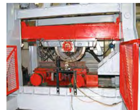
Figure 5.4.1-1: Left: twin disk test rig (SUROS), right: linear test rig (VAS)
