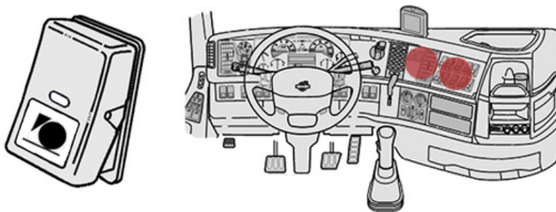
Figure 5-29: sanding control and location on dashboard. Adapted from Driver's Manual FM/FH (Volvo Trucks 1998).
