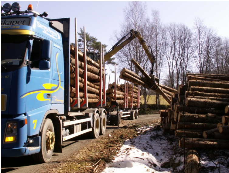
Figure 2-1: using the crane to load timber
