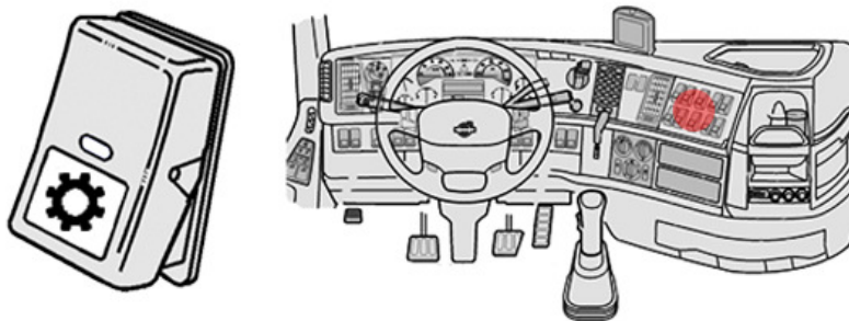
Figure 5-26: Robson-drive control and location on dashboard. Adapted from Driver's Manual FM/FH (Volvo Trucks 1998) .
