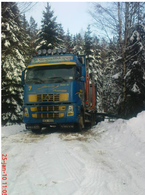
Figure 5-30: a steep slope where sanding was needed but not enough traction was gained
