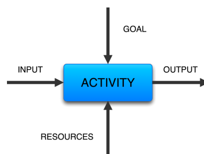
Figure 4.1 Interaction between an activity and elements of product development (O'Donnell and Duffy, 2002)
