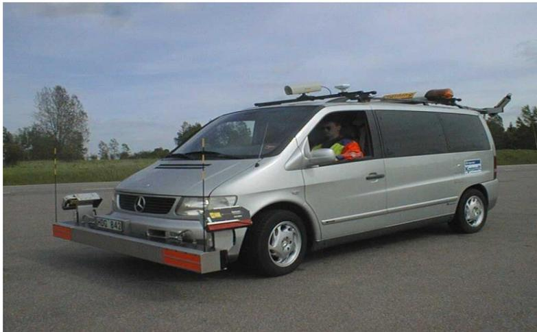
Figure 2.4: RST car used in Sweden (VTI, 2001).
