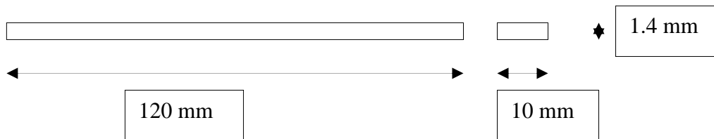
Figure 28 (Nominal dimensions of specimens)
