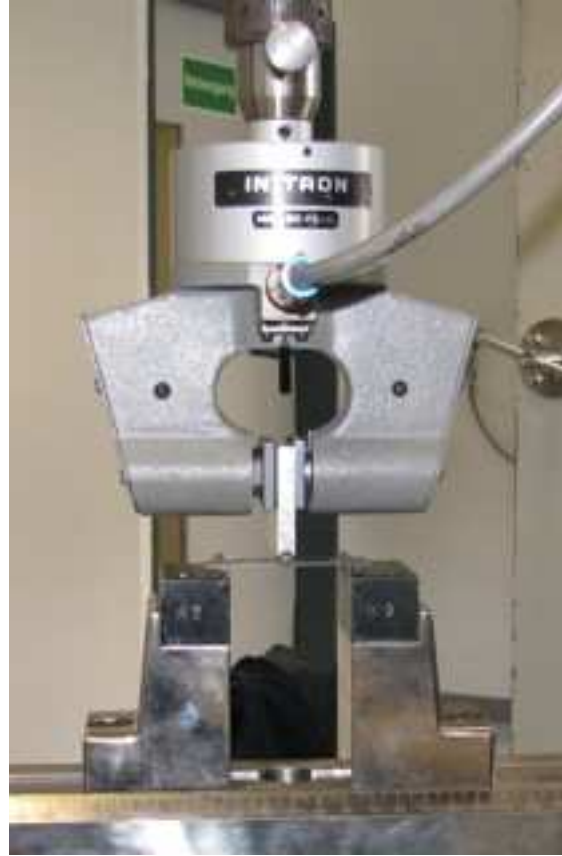
Figure 36 (Setup for 3-point-testing)
