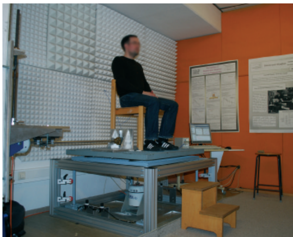
Figure 2.2.: Side view of the Vibration-floor with a seated proband
