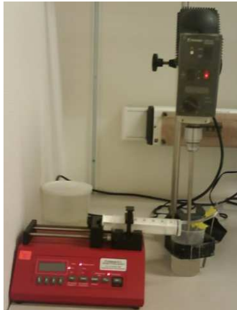
Figure 2: Production of PECs by adding CPAM solution to CMC solution under constant stirring and addition rate.
