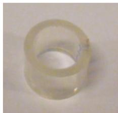
Fig 2.1 Photo of a specimen cut from the hose
