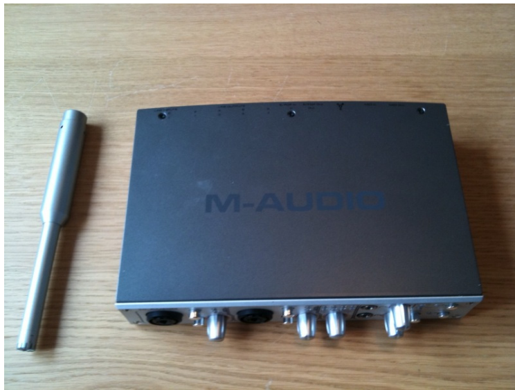
Figure 5.1: Soundcard and microphone used during the measurements.
