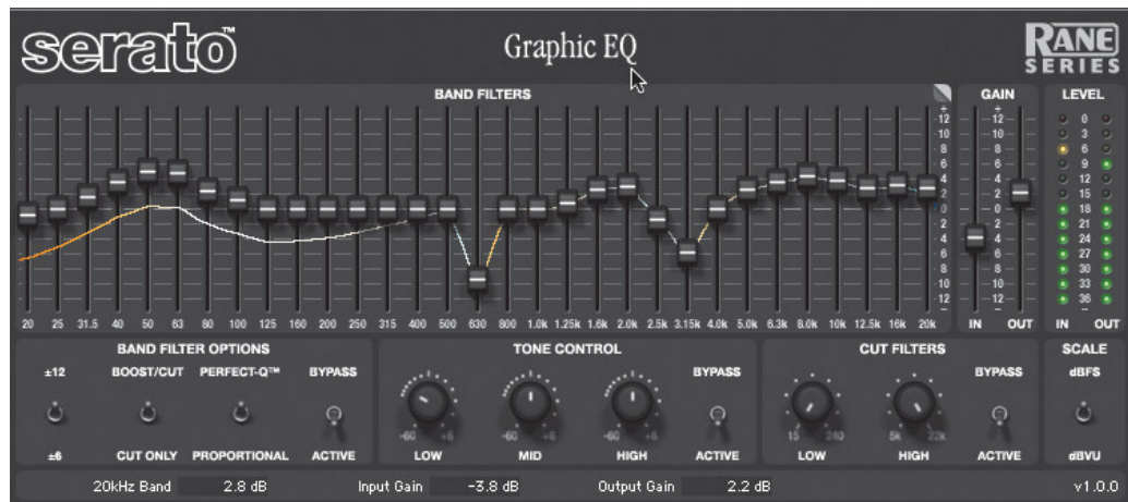
Figure 3.5: A digital implementation of a third octave band graphic equalizer [Ran 10].
