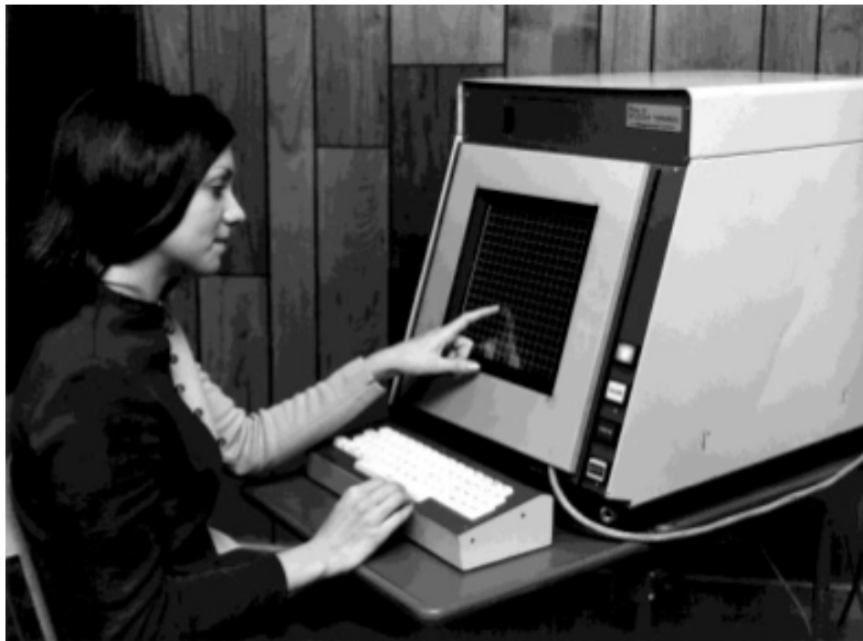
Figure 1: The Plato IV terminal with its touch-sensitive screen [1].
