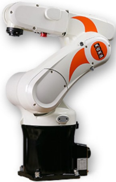
Figure 11: KUKA KR 5 sixx R650 robot with its specifications [13].
