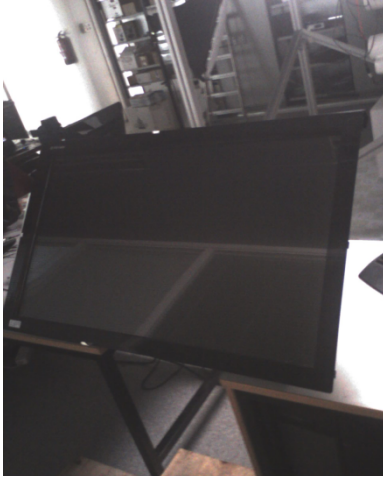
Figure 12: PQ Labs G3 Multi-touch overlay and LG 42" full HD screen [14].
