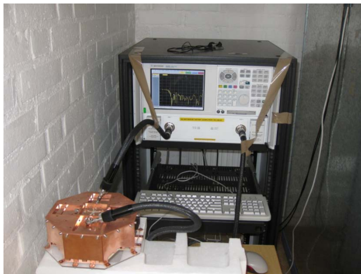
Figure 5: measurement setup using two port of network analyzer
