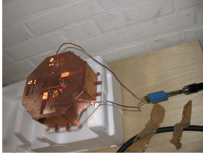
Figure 2: measurement setup using one port of network analyzer
