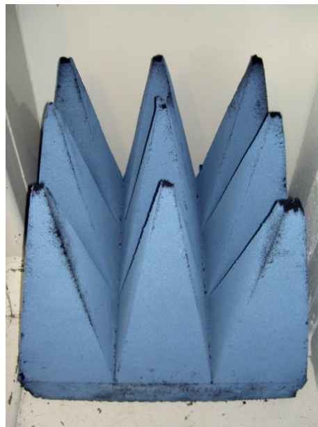
Figure 3.6 The absorber consisting of carbon loaded foam used in the measurements.
