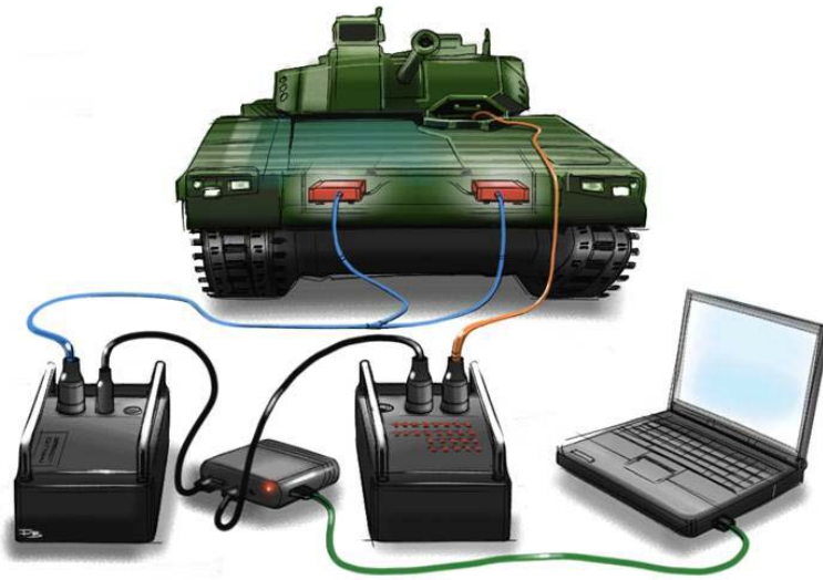
Figure 22. Schematic of DIS connected to a target system
