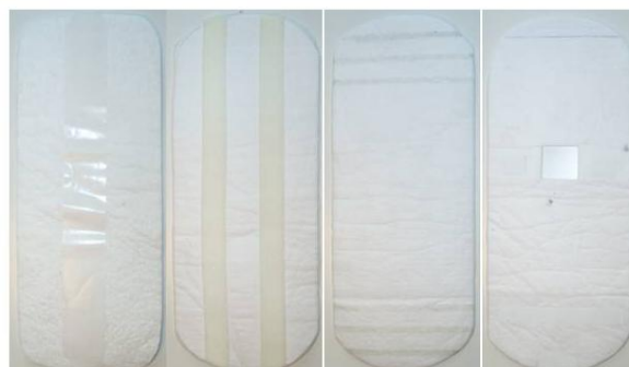
Figure 6.11, Attachments methods; glue with protecting strip, Friction foam, glue and Velcro.
