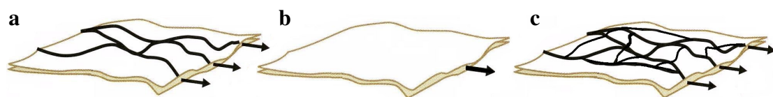
Figure 4.2 a: Fracture with channelled flow. b: Fracture where water spread radially. c: Fracture with enough channels to enable a radial spread of water. Modified from Gustafson (2009).
