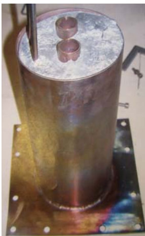
Figure 2.6. The interior of the preheater. The cartridge heater is situated in one of the tubes in the middle, the other one is a preparation for use of two cartridge heaters. The water pipe enters and leaves the aluminum to the left in the picture.
