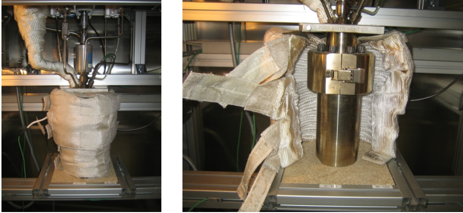
Figure 2.7. The reactor with and without the electrical heating jacket on.
