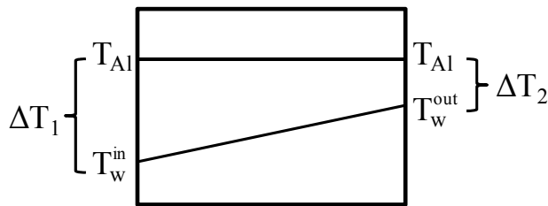
Figure 4.4. The temperature profile for the preheater. The temperature differences used to calculate the logarithmic mean temperature are also indicated in the figure.
