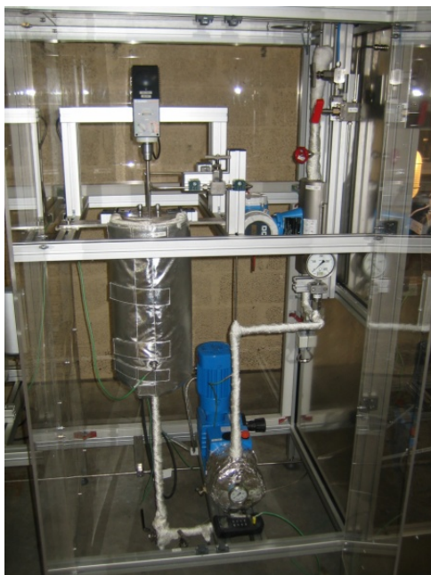
Figure 2.3. The educt box. The storage tank and the pump are the main components of the unit.
