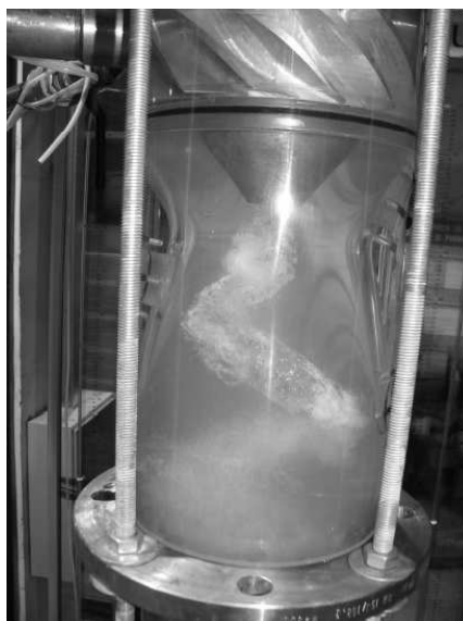
Figure 1.1: A precessing vortex rope, created by the swirling flow in the test rig.
