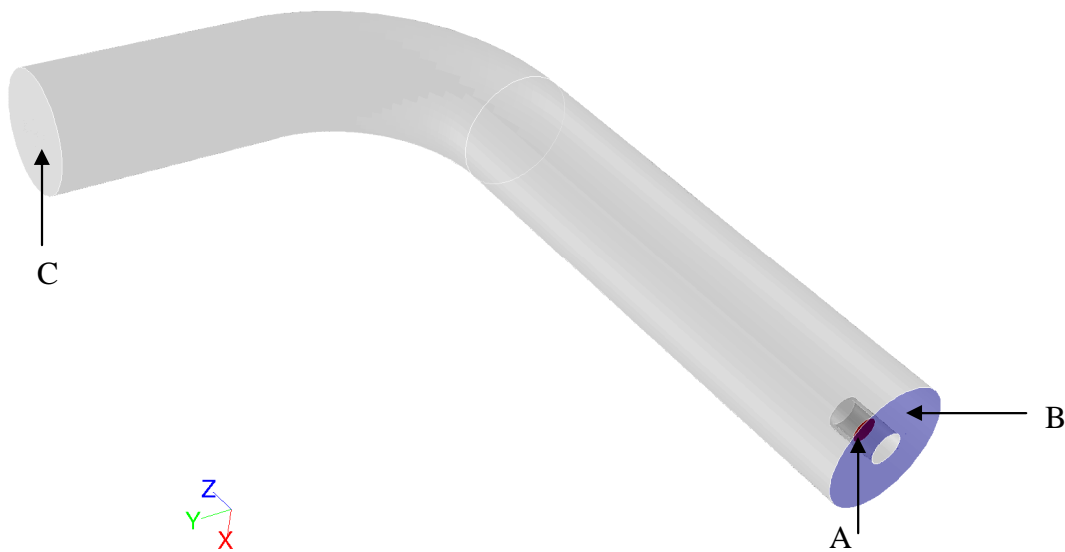
Figure 3.1 Pipe segment used in neutralization of hydrochloric acid using a sodium carbonate solution. In the figure A denotes the acid inlet. B denotes the sodium carbonate solution inlet. C is the geometry outlet.
