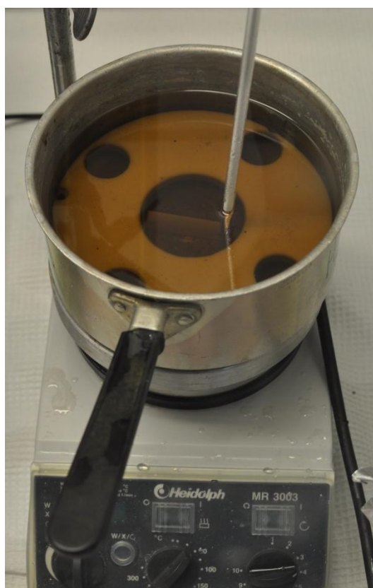
Figure 4 Picture of the equipment used for heating. The headspace vials were placed in the 4 small holes while the big hole allowed the stirrer to rotate freely while staying in the centre. The white rod is the thermometer of the bath. The glycerol has a brownish colour due to berry residue.
