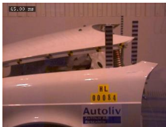
Figure 1-6 Active hood in the lifted position (Fredriksson et al., 2001)
