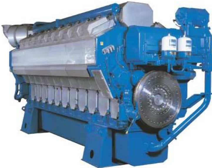
*Figure 4-24: Wärtsilä 34SG engine. By courtesy of Wärtsilä [28][4]*
