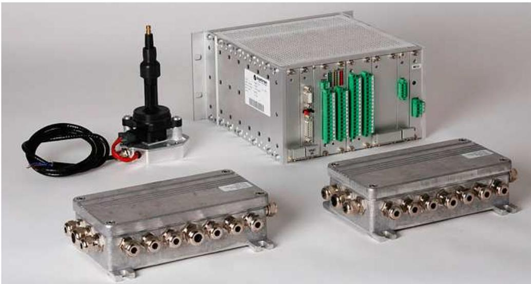
*Figure 1-1: The EMS system. Top left – IU, top right – MC, bottom left – CM and bottom right – KM*
