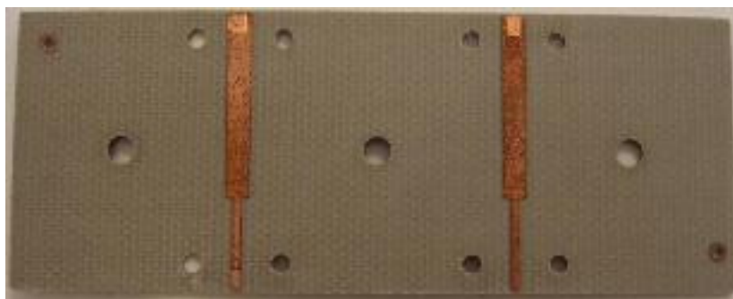
Fig. 4.24 Photo of the transmission lines in manufactured network 1. Antenna ports are on the upper side.
