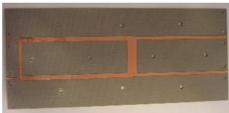
Fig. 4.36 Photo of the transmission lines in manufactured network 3. Antenna ports are to the right.
