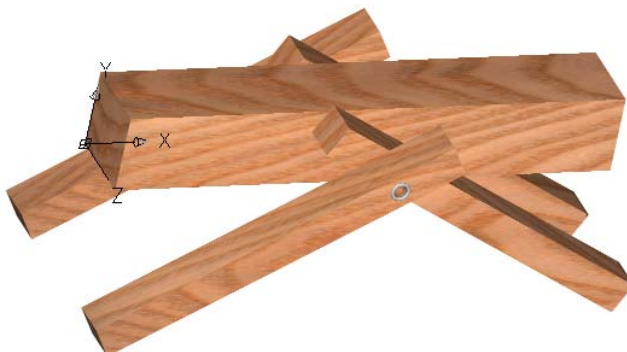
Figure 5.14 Example of truss connection with a tube joint
