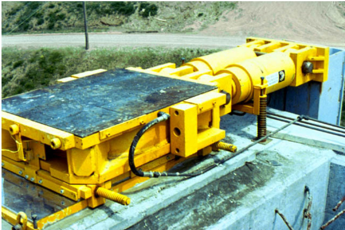
Figure 1.8 A lift-and-push jack. The vertical jack lifts the bridge and the horizontal pistons push the jack forward. Then the vertical jack is lowered and the sledge is retracted and the procedure is repeated.
