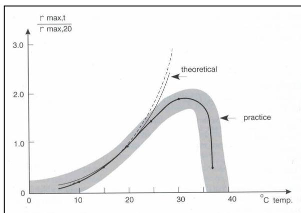
**Diagram 3.3** The nitrification rate's dependency of the temperature, T<sub>0</sub> = 20 °C (Henze et al., 2002).
