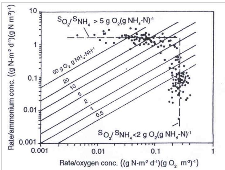
Diagram 4.6 The nitrification rate to ammonium nitrogen concentration ratio as a function of the nitrification rate to oxygen concentration ratio (Hem et al., 1994).
