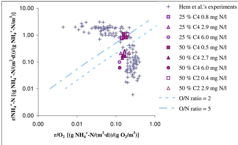
**Diagram 5.5** The nitrification rate to ammonium nitrogen concentration ratio as a function of the nitrification rate to oxygen concentration ratio.
