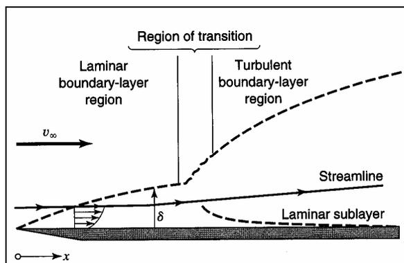
**Figure 3.1** Hydrodynamic boundary layer on a flat plate (Welty et al., 2001).
