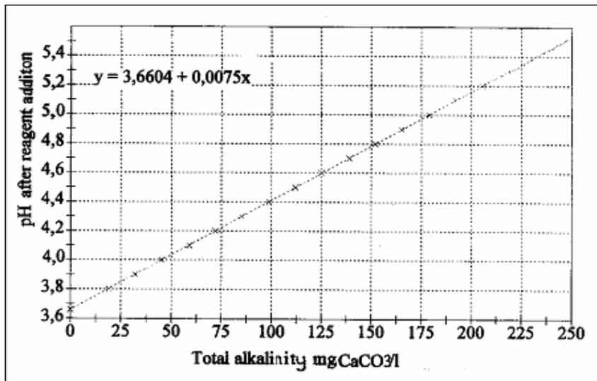
Figure 1. The pH-value after reagent addition plotted against total alkalinity (Robinson, 1994).
