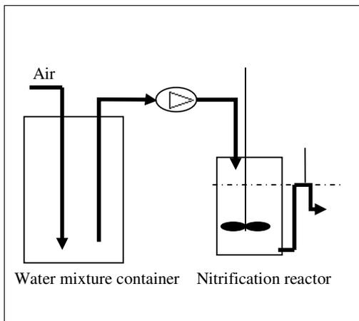
**Figure 4.2** Flowchart of one line in the laboratory-scale plant.
