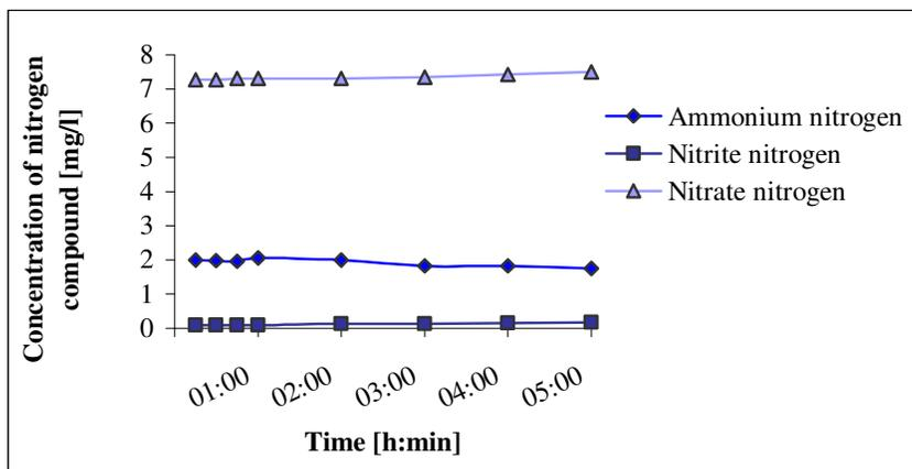
**Diagram 4.2** The nitrogen compounds' concentrations over time for the non-aerated water mixture test.
