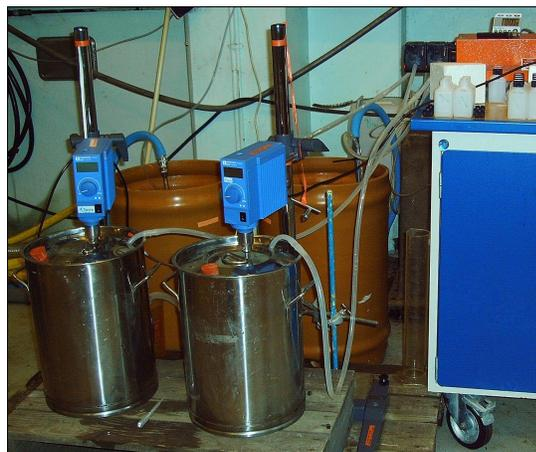
**Figure 4.3** The laboratory-scale plant with the water containers in the back, the nitrification reactors in the front and the pump in the upper right corner.
