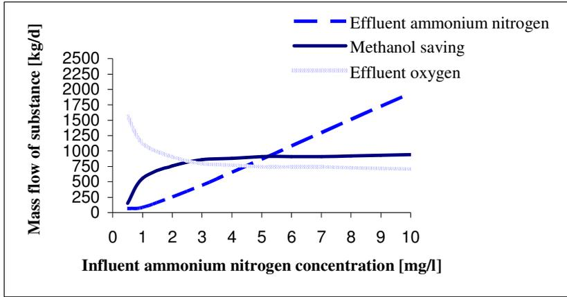
Diagram 4.8 Biofilm area of 240 000 m<sup>2</sup>.
