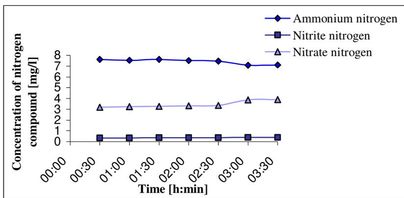
**Diagram 4.3** The nitrogen compounds' concentrations over time for the water mixture in the water container.
