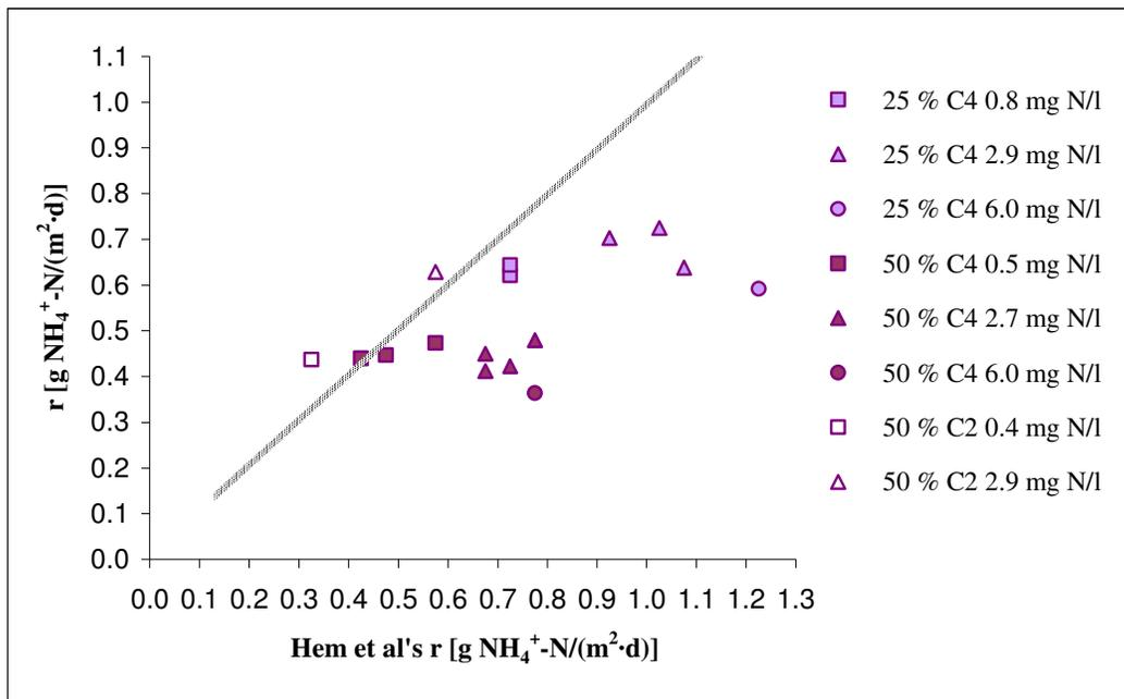
**Diagram 5.6** The obtained nitrification rates from the experiments plotted against Hem et al.'s corresponding nitrification rates (1994).
