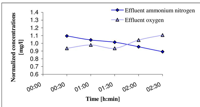
**Diagram 5.1** Effluent ammonium nitrogen and oxygen concentrations for 25 % carrier element filling and low influent ammonium nitrogen concentration.
