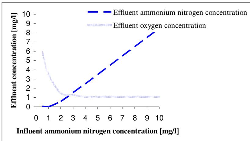
**Diagram 5.10** Biofilm area of 960 000 m<sup>2</sup>.
