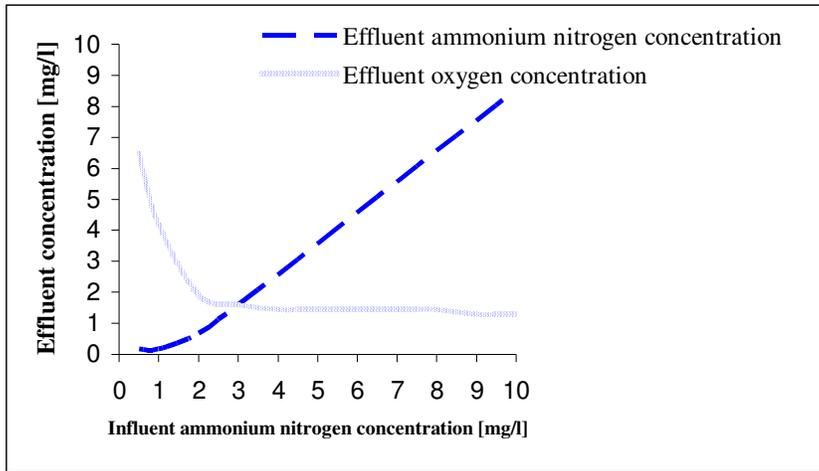
**Diagram 5.9** Biofilm area of 720 000 m<sup>2</sup>.
