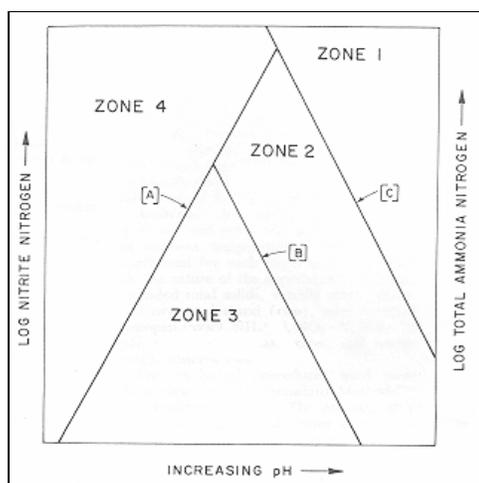
**Diagram 3.2** Relationship of ammonia and nitrous acid inhibition to nitrifying bacteria (Anthonisen, et al., 1976).
