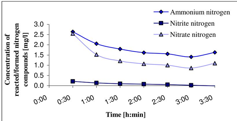
Diagram 4.5 Reacted ammonium nitrogen and formed nitrite and nitrate nitrogen in the nitrification reactor.
