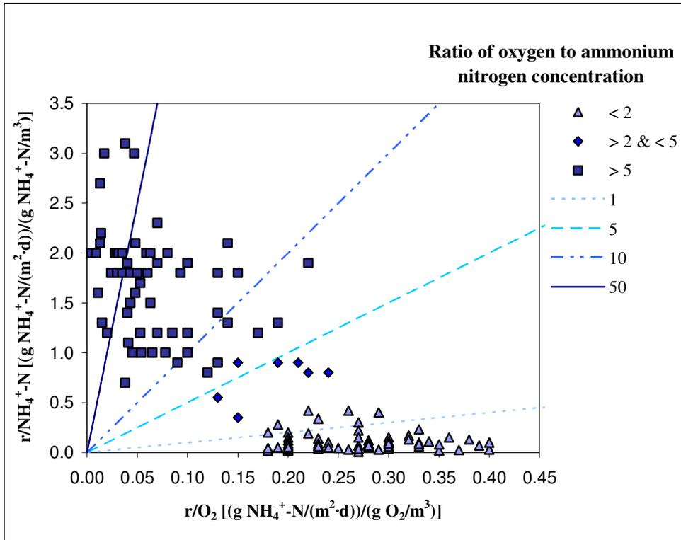
**Diagram 4.7** The nitrification rate to ammonium nitrogen concentration ratio as a function of the nitrification rate to oxygen concentration ratio.
