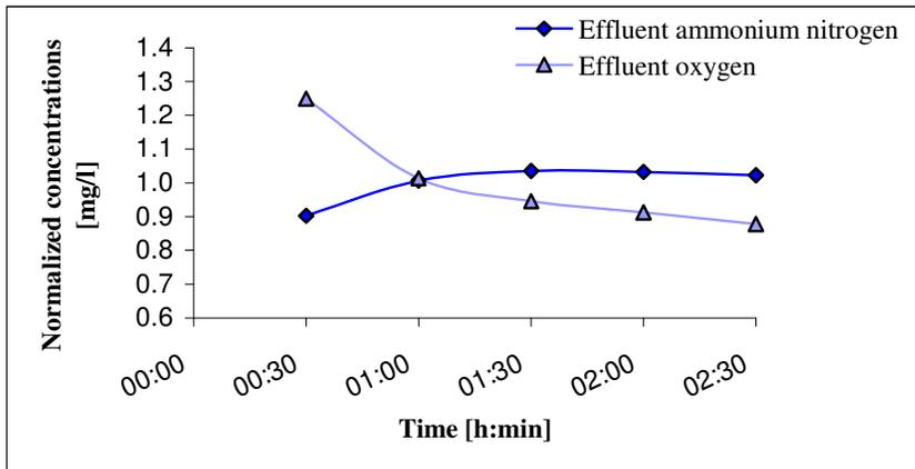
**Diagram 5.4** Effluent ammonium nitrogen and oxygen concentrations for 50 % carrier element filling and high influent ammonium nitrogen concentration.
