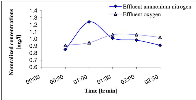
**Diagram 5.3** Effluent ammonium nitrogen and oxygen concentrations for 50 % carrier element filling and low influent ammonium nitrogen concentration.
