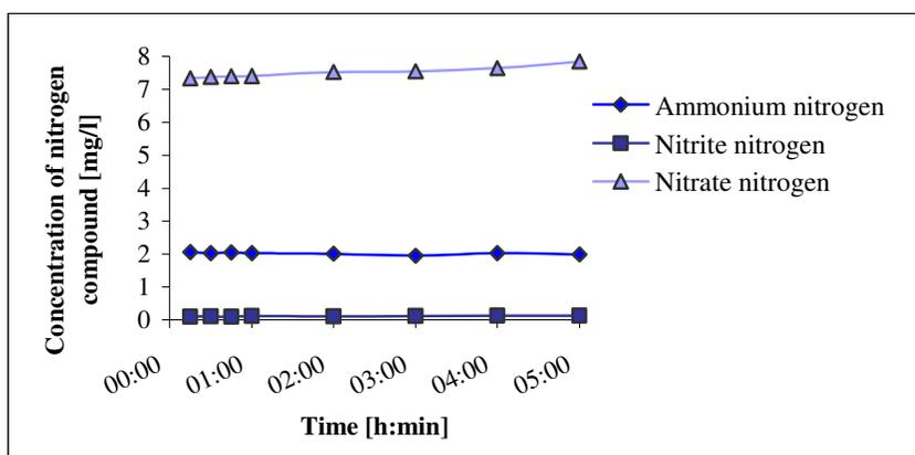
**Diagram 4.1** The nitrogen compounds' concentrations over time for the aerated water mixture test.
