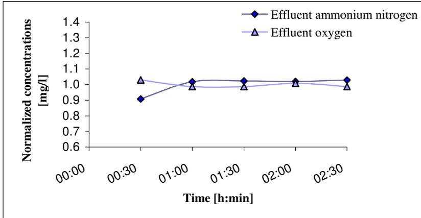
**Diagram 5.2** Effluent ammonium nitrogen and oxygen concentrations for 25 % carrier element filling and high influent ammonium nitrogen concentration.
