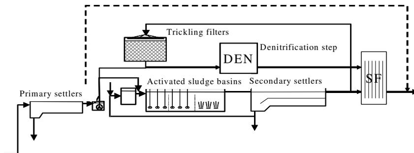
**Diagram 1.2** Flowchart of the planned water purification process.
