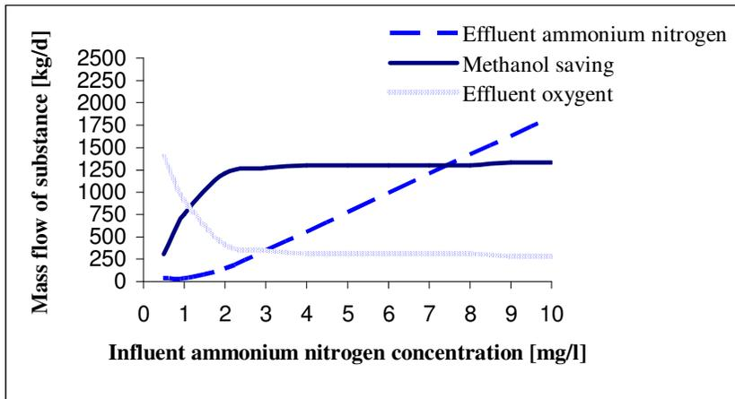
Diagram 4.10 Biofilm area of 720 000 m<sup>2</sup>.
