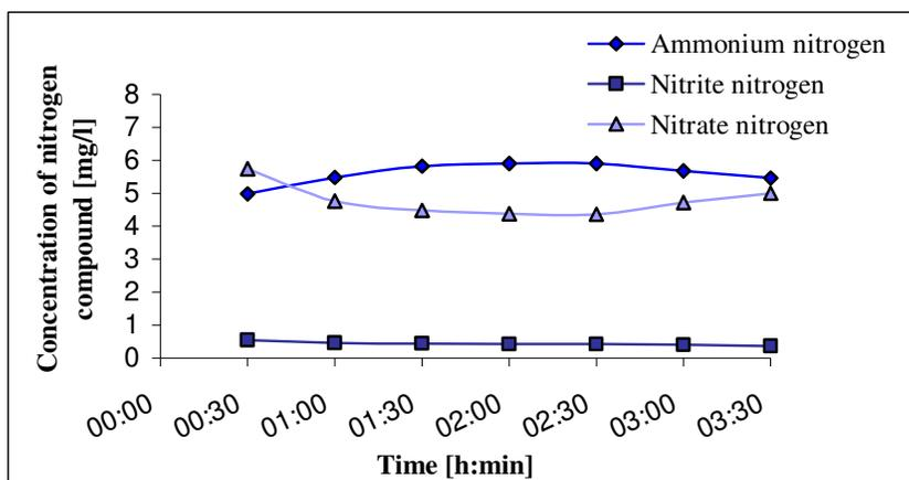
**Diagram 4.4** The nitrogen compounds' concentrations over time for the water mixture in the nitrification reactor.
