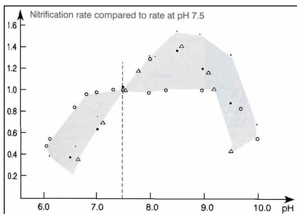
**Diagram 3.1** The nitrification rate's dependency of the pH (Henze et al., 2002).
