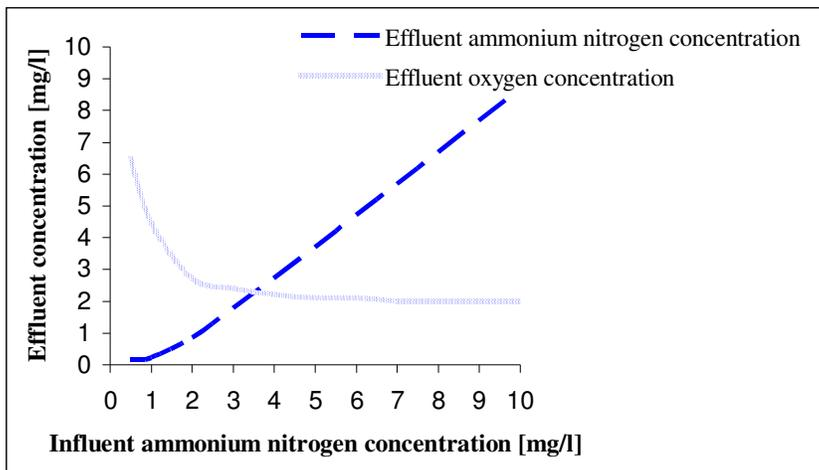
Diagram 5.8 Biofilm area of 480 000 m<sup>2</sup>.
