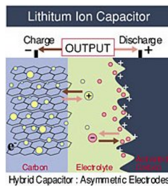
Figure 2.20: Structure of a Li-ion capacitor, [22]
