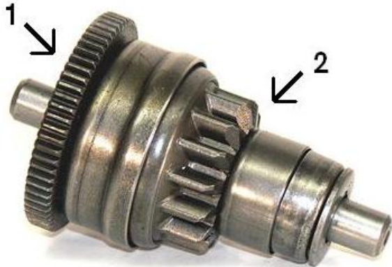
Figure 6, Piaggio bendix gear used to connect start motor to the ICE [6]
