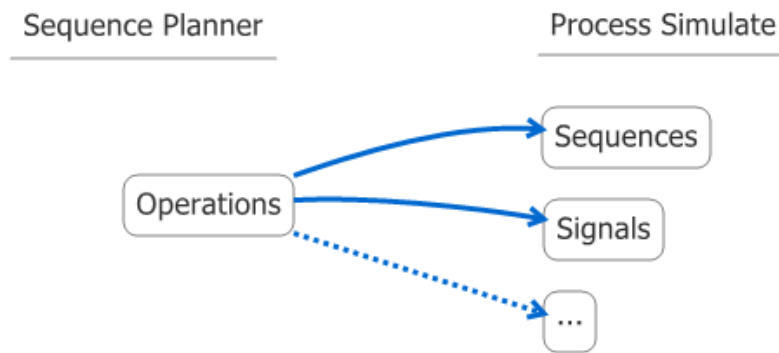
Figure 5.9: Difference between data types between Sequence Planner and Process Simulate.
